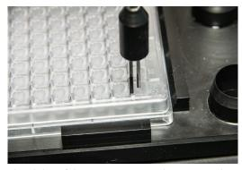
The ability of the REMS AutoSampler to precisely locate the electrode results in highly reproducible TEER measurements.
