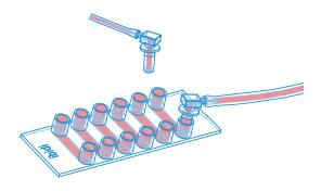
4. Open the clamped tubing and conduct your perfusion experiment.
